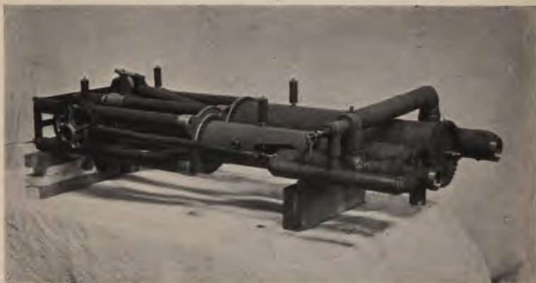
Fig. 85.—One pair of my compound engines. This engine weighed 310 lbs. and developed 180 H.P., with 320 lbs. of steam per square inch.
